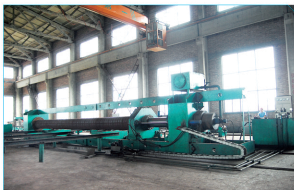
Hydrostatic testing/水压试验
