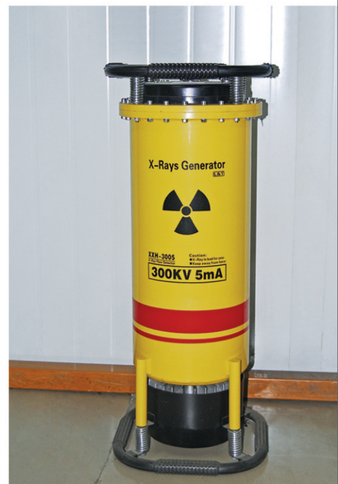
□ X-rays generator/X射线检测
